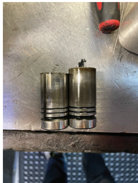
The worn down tappet on the left hand side, and on the right. a good hydraulic tappet.
