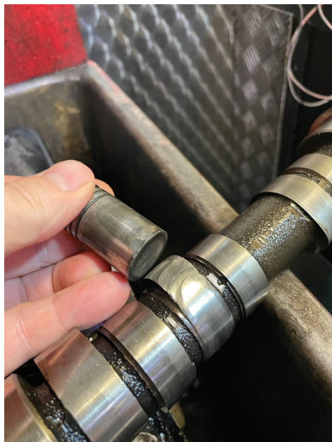
The worn camshaft lobe and worn down hydraulic tappet.
